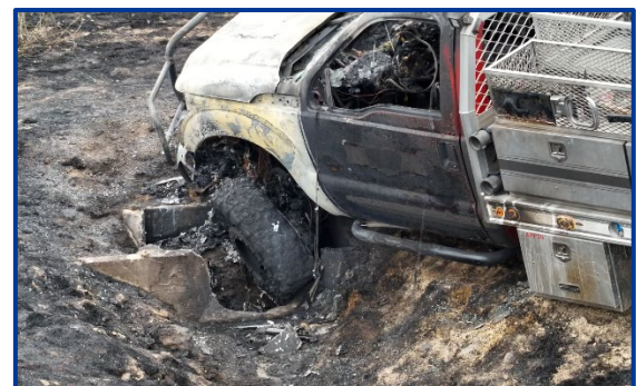
The abandoned irrigation canal—that could not be seen from the engine's cab—that immobilized the engine.
